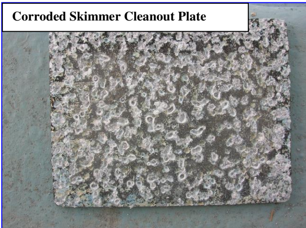
Corroded Aluminum Fitting
